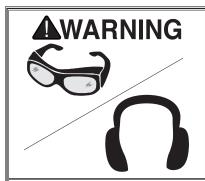
Operating this nailer can propel objects into the air, causing immediate eye damage. To protect yourself, always wear ANSI approved safety glasses or goggles when operating this equipment.
